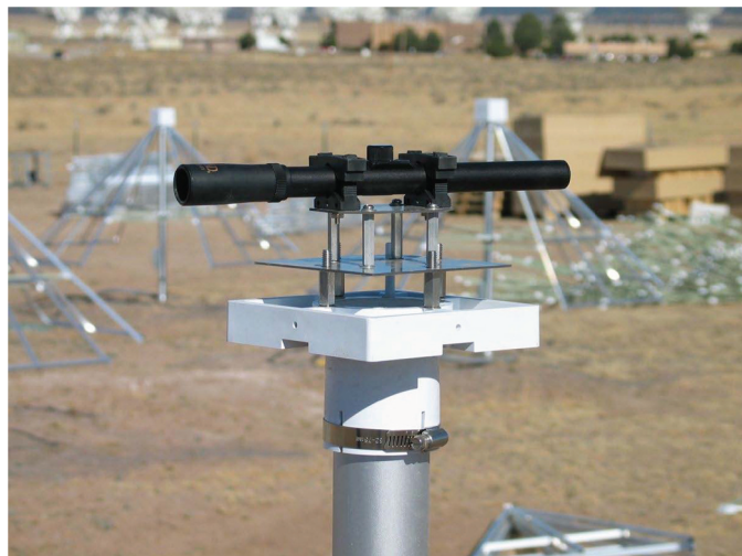
FIG. 10.—STD sighting telescope alignment mechanism used for the LWA1. See the electronic edition of the PASP for a color version of this figure.
